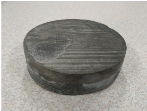
Figure 2: A cylindrical sample of a hardened cement slurry with a rubber powder additive.
