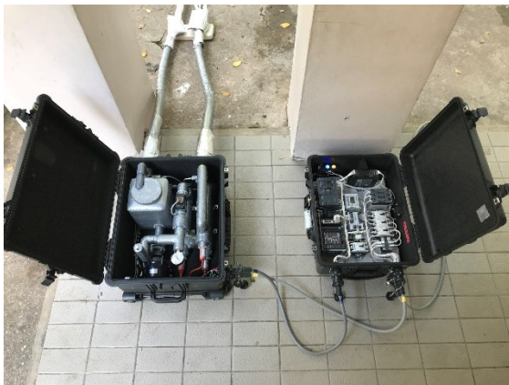
Figure 7. TRT measurement in Bangkok GSHP site
