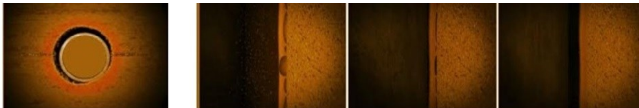
Figure 2: Plastering effect during CwD (modified from IADC 2015)
