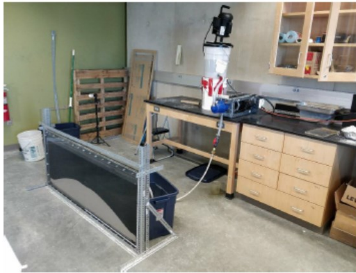
Figure 1: The experimental setup consisting of buckets for proppant mixing with motorized mixer, a motorized progressive cavity pump and acrylic-aluminum narrow fracture cell.
