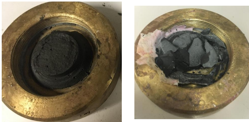
Figure 9. The bottom part of the shear test cell after testing at 24 hours (left) and 82 days (right)
