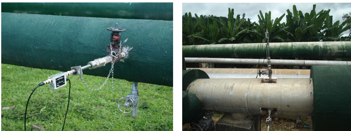
Figure 2: RF sensor installed through standard TFF injection port, and second sensor installed at sample port.
