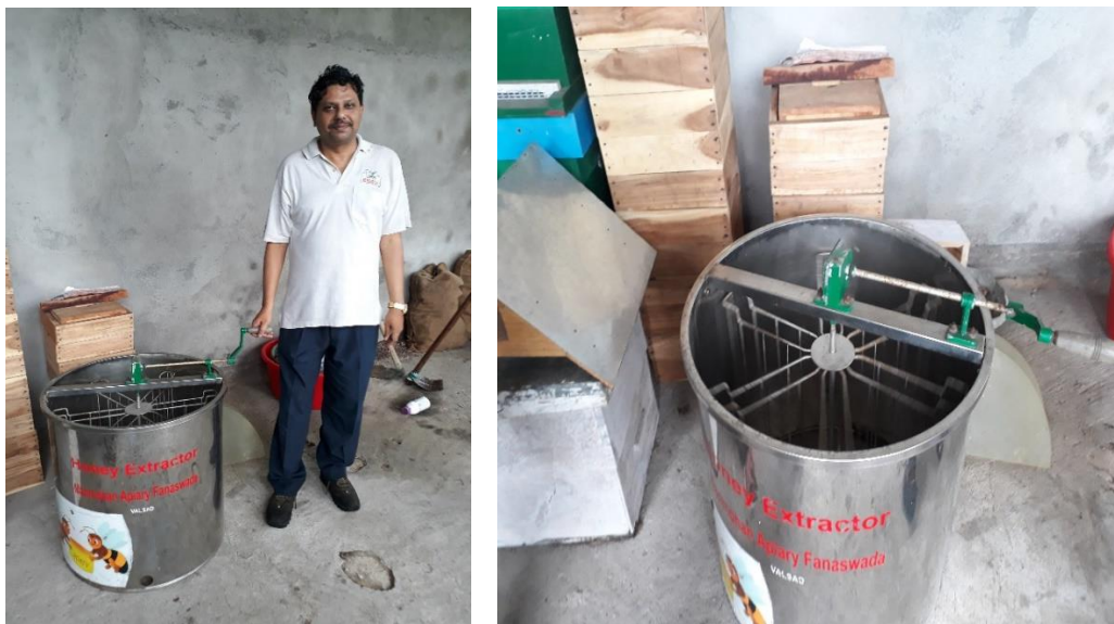
Figure 3: Centrifugal manually driven (hand crank) 6 frame honey extractor
