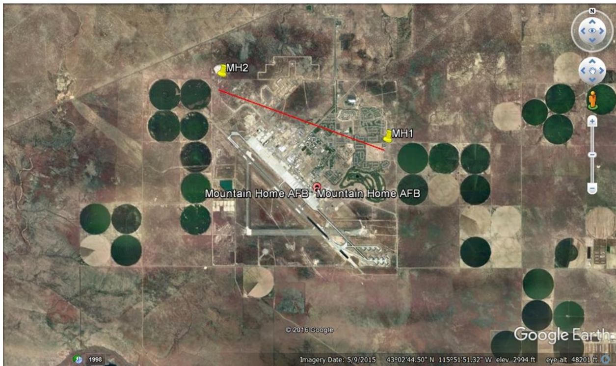
Figure 1. Image of Mountain Home AFB showing the locations of MH-1 and MH-2. The red line shows the surface projection of the hydrothermal fault penetrated by drilling in MH-2 that is also consistent with lithologic logging of MH-1 (Lewis and Stone, 1988).
