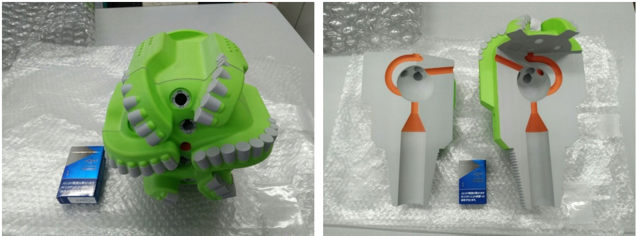
Figure 10: Prototype 3D printed model of the 8-1/2" thermal-shock enhanced drill bit.
