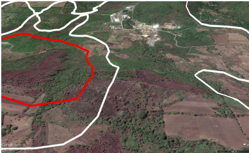
Figure 13: View of El Tizate production area looking eastwards and down slope into the El Tizate production area valley from the rim of the Los Tablones fault. Recharge flows down toward El Tizate from Los Tablones and the higher elevation catchment to the west. Recharge forms a reservoir at the El Tizate topographic low; note the hill immediately to the east of the production area prevents recharge escaping further east. Recharge is heated and acidified (by CO 2 , H 2 S), and alters volcanics to clay. White boundary is the LFZ that results from the clay cap. Red boundary encloses HFZ to the north, located on adjacent catchment. Image with vertical exaggeration from Google Earth.
