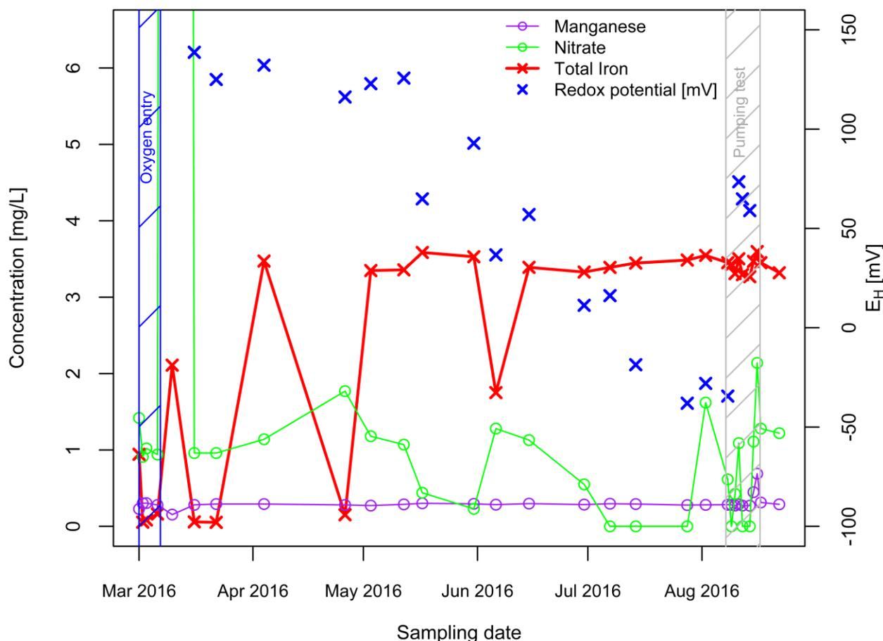
**Figure 2:** Long-term course of redox-sensitive parameters at Berlin-Southwest site between start of operation in March 2016 and end of tracer test in August 2016. Oxygen entered the system accidentally for 5 days in continuous operation in March 2016. A pumping test was conducted in August 2016 for 10 days.
