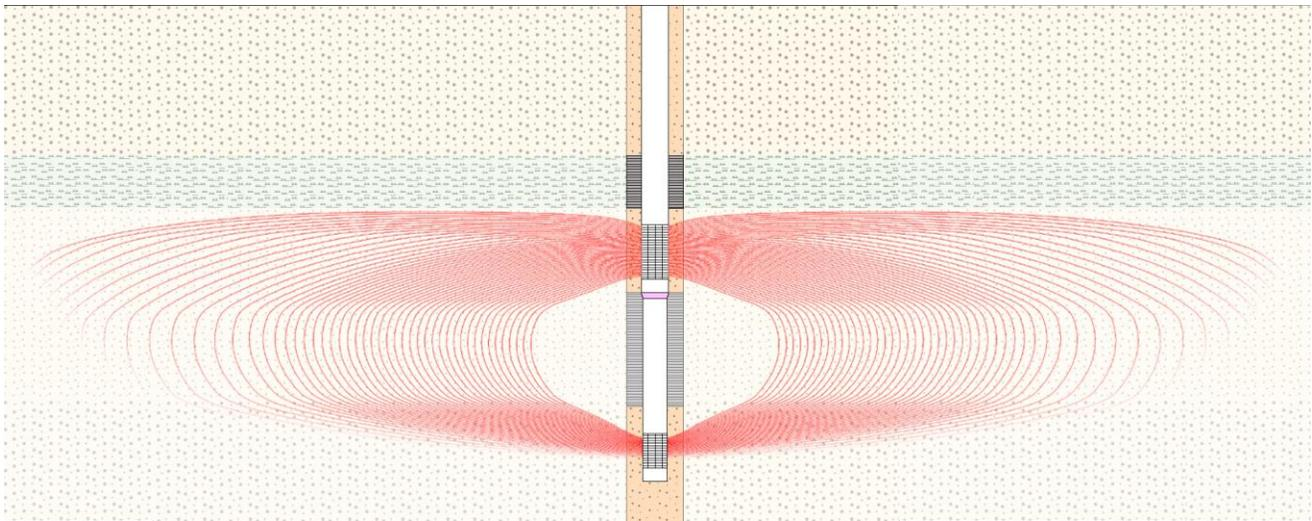
**Figure 1: Modeled circulation cell of re-injected groundwater from upper filter screen to lower filter screen. The depicted GCW is located at Berlin-Southwest site at pumping rate  $8.6 \text{ m}^3/\text{h}$  without groundwater flow with FeFlow 6.1. The vertical expansion of the circulation cell is 40 m assuming a continuous pumping time of more than 100 days. Real operation cycles are less than four hours per day.**
