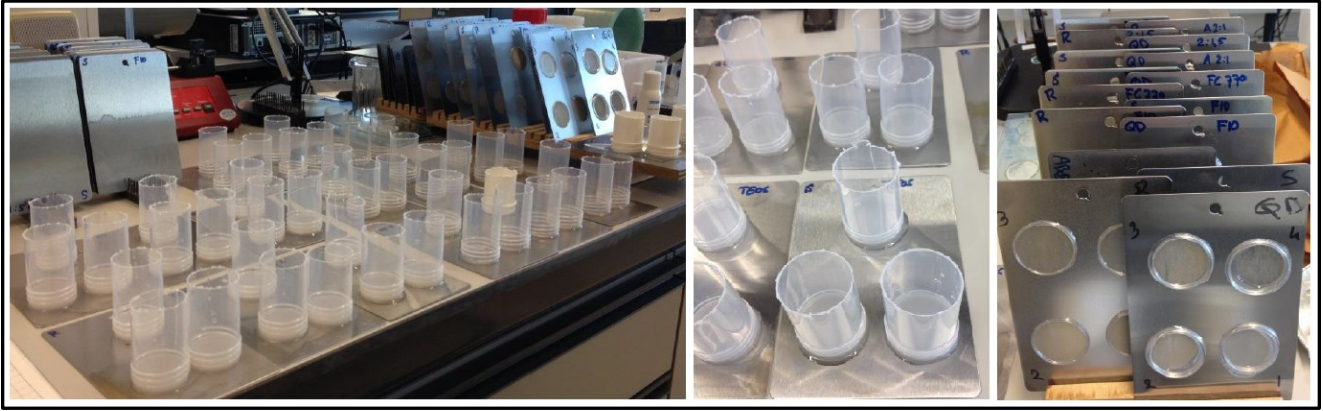
Figure 2. Large scaling experiments on 30 different substrate-surface modifier combinations. Left: overview. Center: samples during scaling. Right: samples after scaling.
