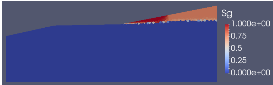
Figure 7: Gas saturation at final time (1000 years) obtained with the evaporation-outflow boundary condition.
