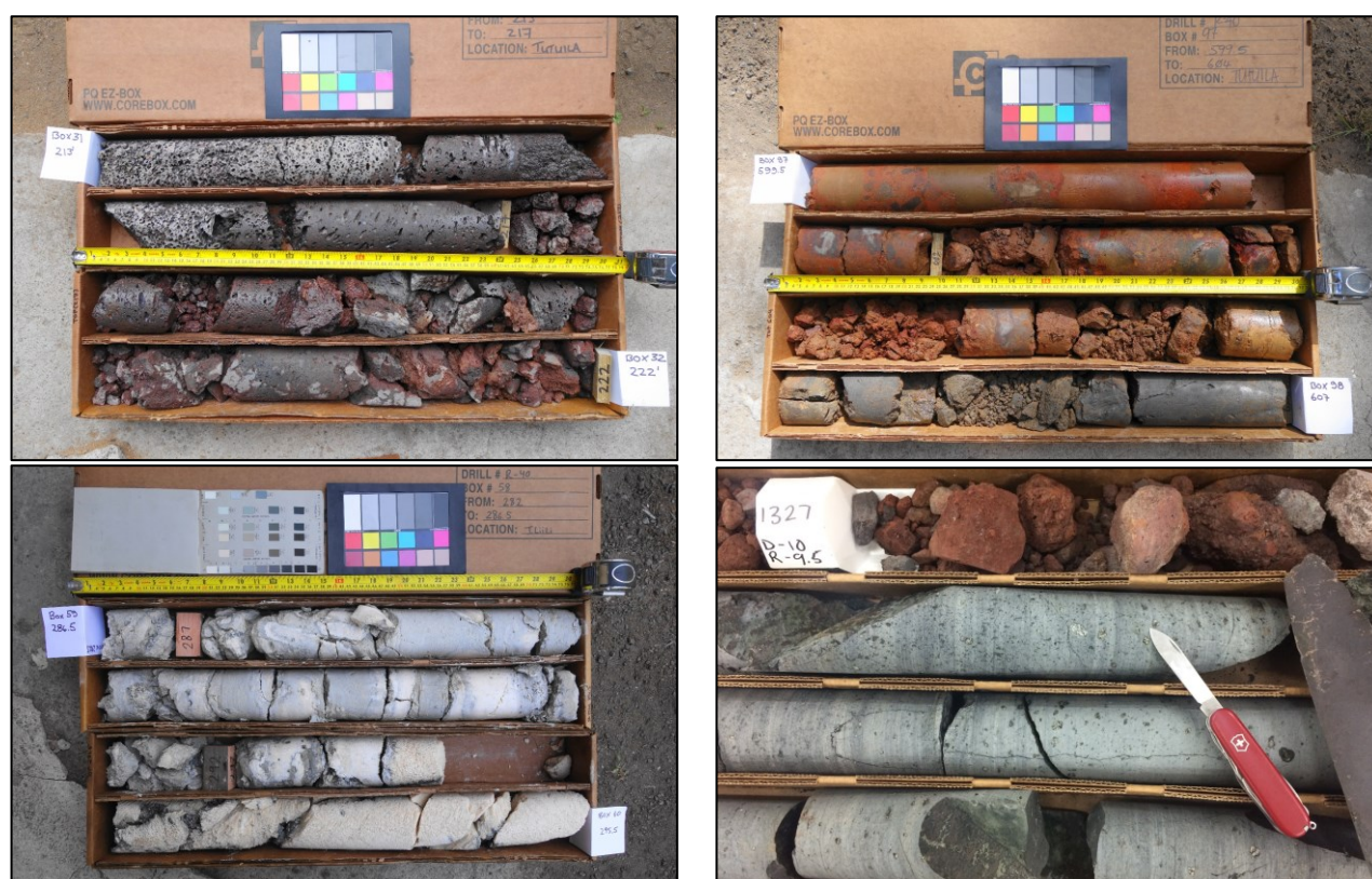
Figure 10. Lithology from the two TGH. Top Left: Young Leone Volcanics basalt flows from ~ 220 ft bgs (TGH-1). Top Right: Taputapu Volcanics debris flow at ~600 ft bgs, highly altered by Fe-clays and hematite (TGH-1). Bottom Left: Leone Carbonates reef structures at 295 ft bgs (TGH-3). Bottom Right: Taputapu Volcanics olivine basalt at 1329 ft bgs (TGH-3).
