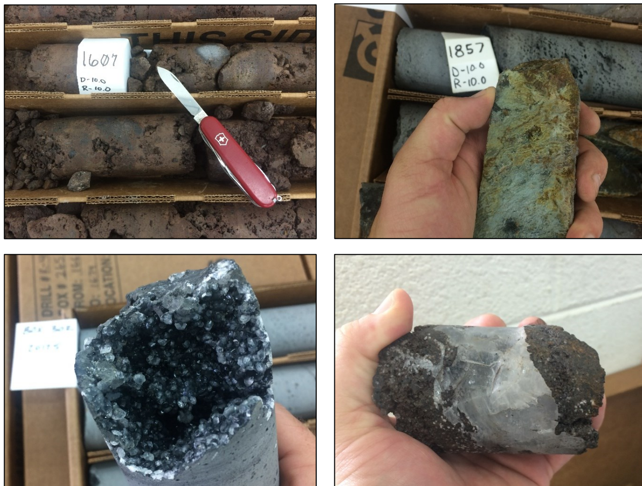
Figure 12. Details of core. Top Left: Brown limonite alteration of clay-rich volcanoclastic at 1,607 ft bgs in TGH-3 Top Right: Kaolinite-serpentine clays coating high-angle fracture at 1,860 ft in TGH-3. Bottom Left: Dog-tooth zeolite crystals at 2,021 ft bgs in TGH-3. Bottom Right: Massive gypsum megacryst filling open space at 2,097 ft bgs in TGH-3.
