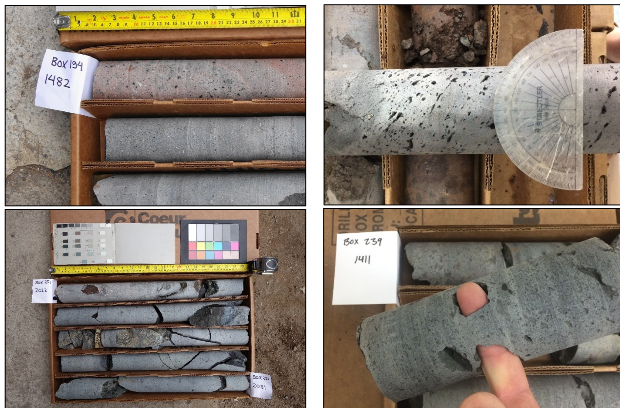
Figure 11. Details of structure in the core. Top Left: Horizontal flow banding at 1,482 ft bgs (TGH-1). Top Right: Dipping vesiculated bedding planes in lava flow (TGH-3). Bottom Left: Fractured lava flow with high-angle fractures and dip-slip slickensides at ~2,030 ft bgs (TGH-1). Bottom Right: High porosity in vesiculated lava flow at 1,413 ft bgs (TGH-3).
