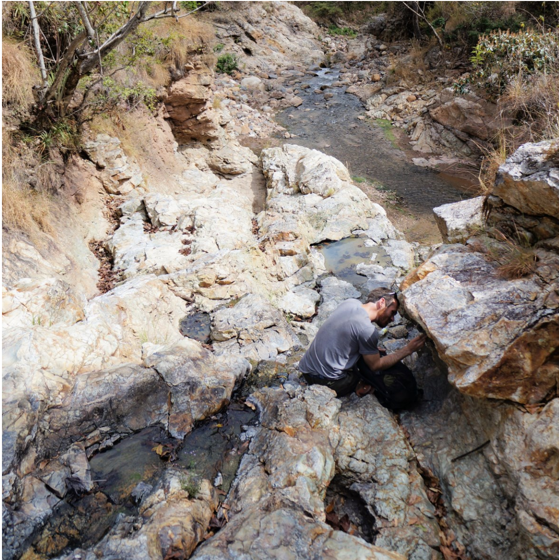
Figure 3 - Field measurements of the Waterfall Fault in silicified Padre Miguel Tuff formation, looking southeast. Hot springs can be seen issuing from the fault zone at bottom right.
