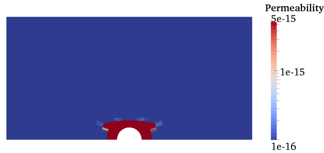
Figure 10. Permeability values around injection well for the Mazars/Pijauder-Cabot initiation criterion. The area of enhanced permeability is localized around the injection site because permeability only increases at higher values of damage/strain as seen in Figures 3 and 5.
