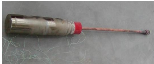
Figure 2: Picture of Heat-pipe prototype connected with PCM-container
