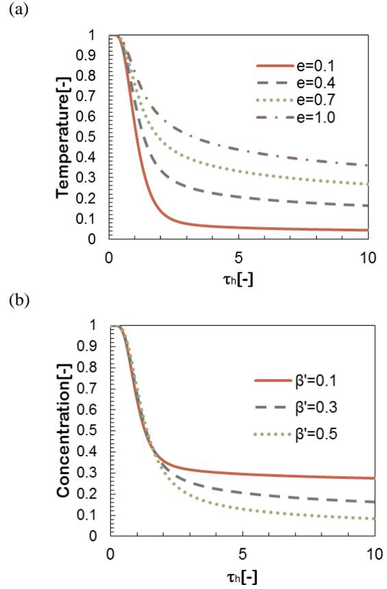
Figure 3. Temperature profiles corresponding to conduction into a surrounding rock. Results and Discussion
