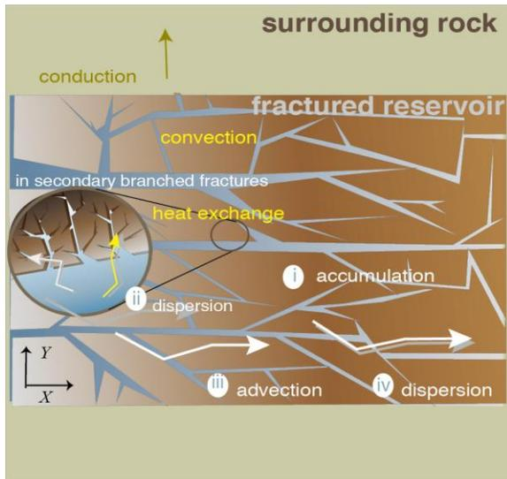
Figure 1: Schematic of a reservoir.
