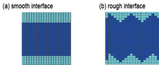
Figure 5: Simulation model to evaluate the effect of cold water injection
