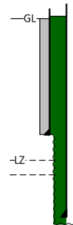
Figure 4: Entire annular space is now filled with good cement, free of contaminants, and job is successfully completed.
