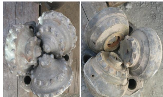
Figure 7. Average bit condition after 300' of typical air drilling in the normal temperature Geysers reservoir (left) and Prati 32 final bit condition after 100' of air drilling to final depth (11,134') in the high temperature reservoir.
