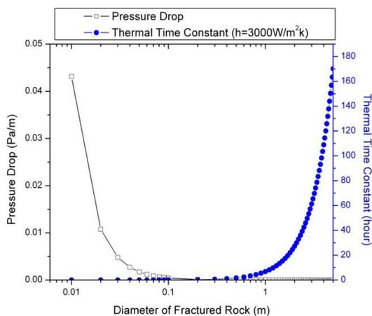
Figure 6: Pressure drop and thermal time constants for the mining option (Lee, Forsberg, Driscoll, Sapiie, 2010)
