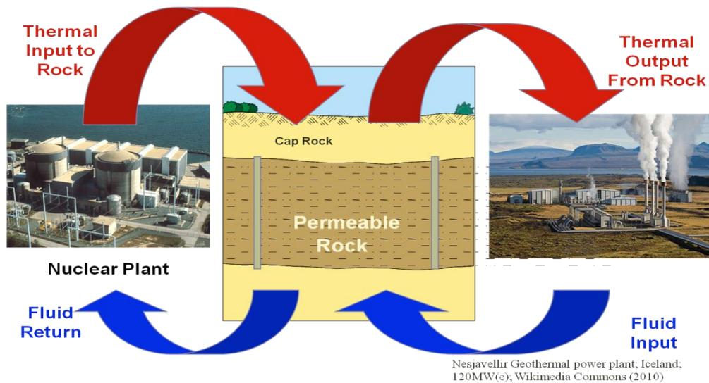
Figure 1: Conceptual Diagram of Nuclear-Geothermal Energy Storage System
