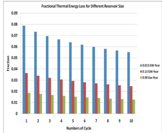
Figure 3: Fractional Heat Losses versus Number of Cycles for Different Size Systems (Lee, Forsberg, 2011): Inlet Temp: 250°C; Outlet Temp: 30°C; Porosity: 0.2; Diameter/Length 0.331, Cycle length: 6 months
