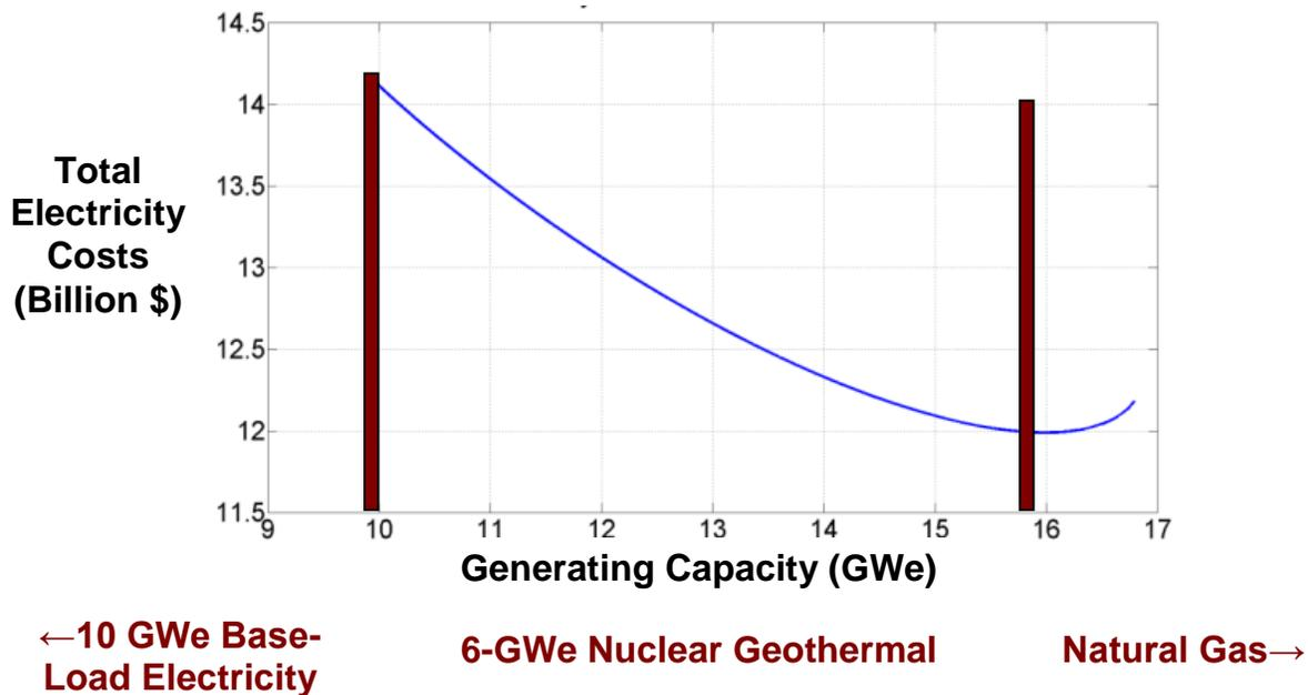
Figure 8: Total Cost of New England Electricity Vs Capacity of Nuclear Geothermal Capacity.
