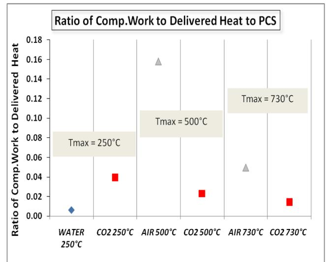
Figure 4: Ratio of Compressor (Pump) Work to Delivered Heat to the Power Conversion System
