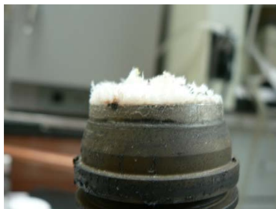
Figure 5. Side view showing the formation of calcium carbonate at the entrance of the flow cell
