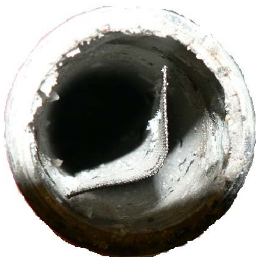
Figure 2. \text{CaCO}_3 crystals formed within the flow cell during an experiment at 190^\circ\text{C} .
