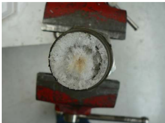
Figure 6. Top view showing the formation of calcium carbonate at the entrance of the flow cell
