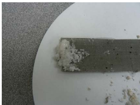
Figure 3. \text{CaCO}_3 crystals that formed at the bottom of the reactor on a metal screen at 190^\circ\text{C} .
