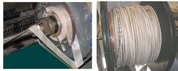
Figure 5. Application of prepreg tape insulation to copper wire (left) and spool of insulated wire (right).
