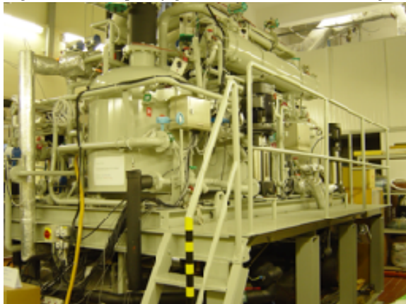
Figure 5: A prototype lab-scale multi-bed adsorption chiller (designed by Assoc. Prof. Hui Tong Chua and Dr. Xiaolin Wang).
