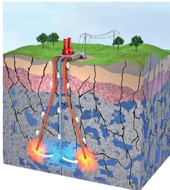
*Figure 1: The Soultz geothermal triplet. Geothermal fluid is pumped by down-hole pumps from 2 lateral production wells (in red), delivering the geothermal energy to a binary power plant on surface. Cooled water is re-injected in the fractured granite by a central injection well (in blue).*
