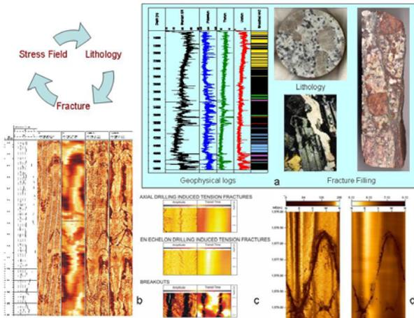
Figure 4. Main geological investigations carried out from well data at Soultz: lithology and hydrothermal alteration from spectral gamma ray and core studies (a), fracture geometry and in-situ stress field conditions (b, c, d).
