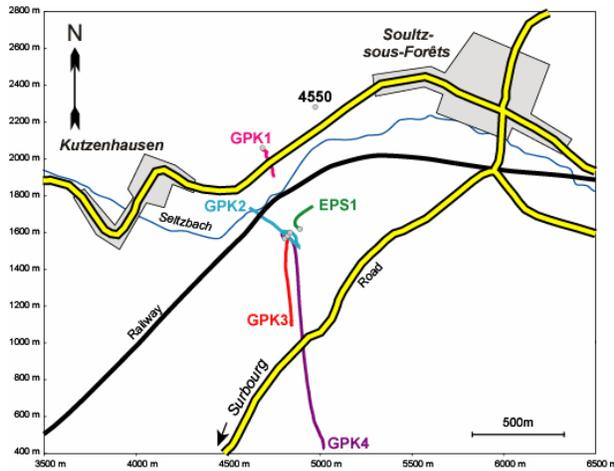
Figure 2. Local map view of the Soultz site between Kutzenhausen and Soultz. 4550 is a seismic well. GPK1 and EPS1 are former exploration wells.
