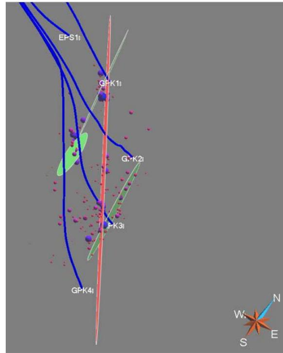
Figure 6. Examples of major 3D planar structures derived from borehole data (red) and microseismicity (green). Well trajectories are plotted in blue from Sausse et al., 2009.
