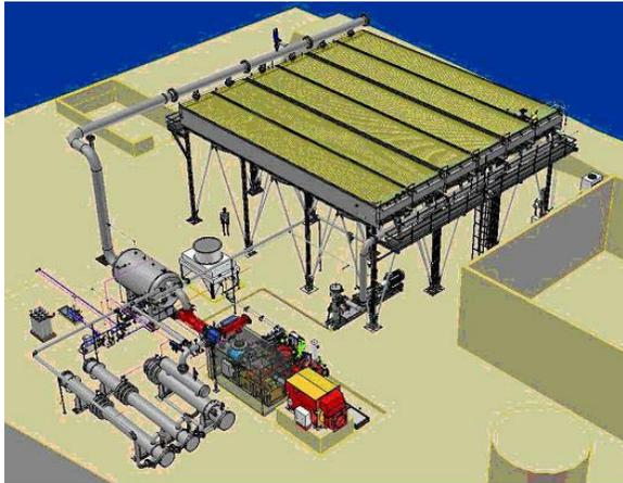
Figure 7. The Soutz ORC unit designed by Cryostar and Turboden.
