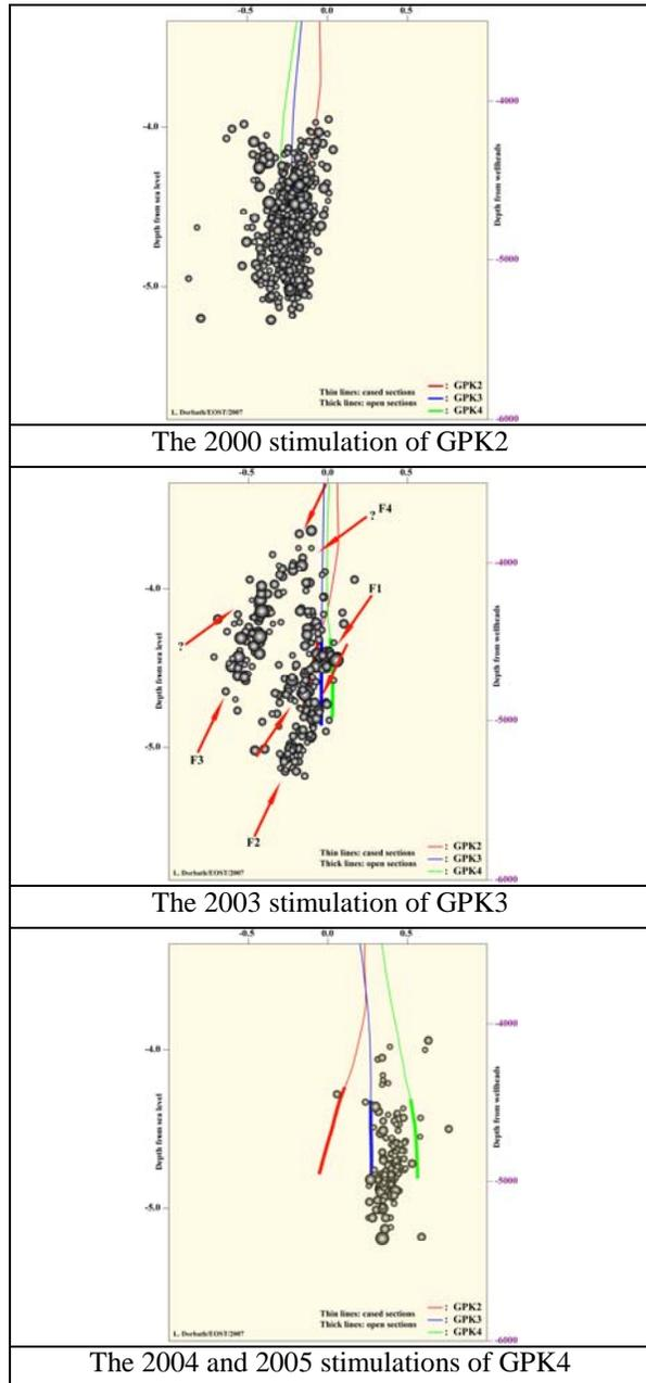
Figure 5. Hydraulic stimulations in the Soultz wells. Seismic clouds of ( $M > 1$ ) events are plotted on nearly N-S cross-sections from Dorbath et al., 2009.
