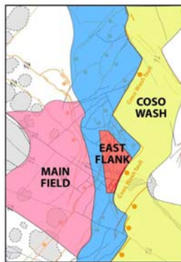
Fig. 1: Fault-controlled sub-divisions of the Coso geothermal area. These are distinct as regards temperature and seismicity. The Main Field and the East Flank are the primary producing and seismically active regions.
