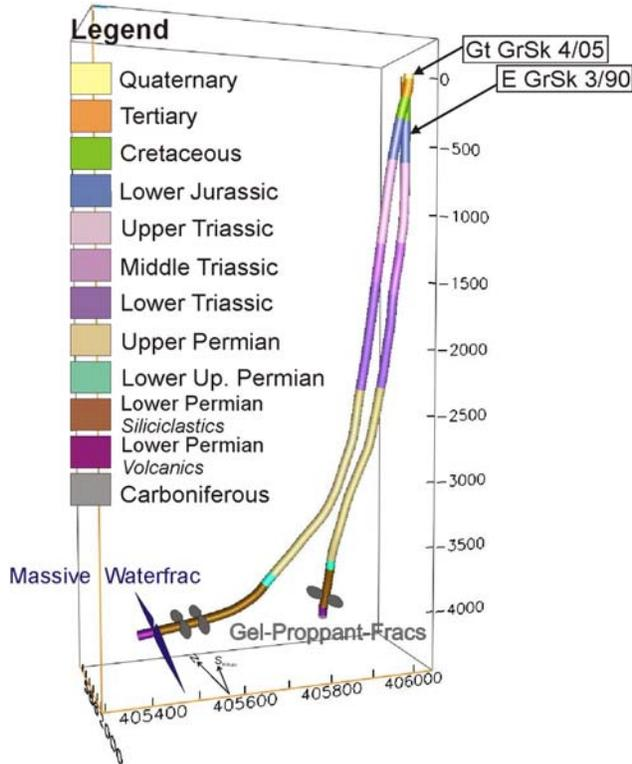
Figure 1 Alignment of the well path and the fracture treatments of the doublet system at the Groß Schönebeck drill site.
