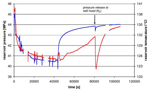
Figure 5 Schedule of the production test including the shut-in with pressure and temperature response.
