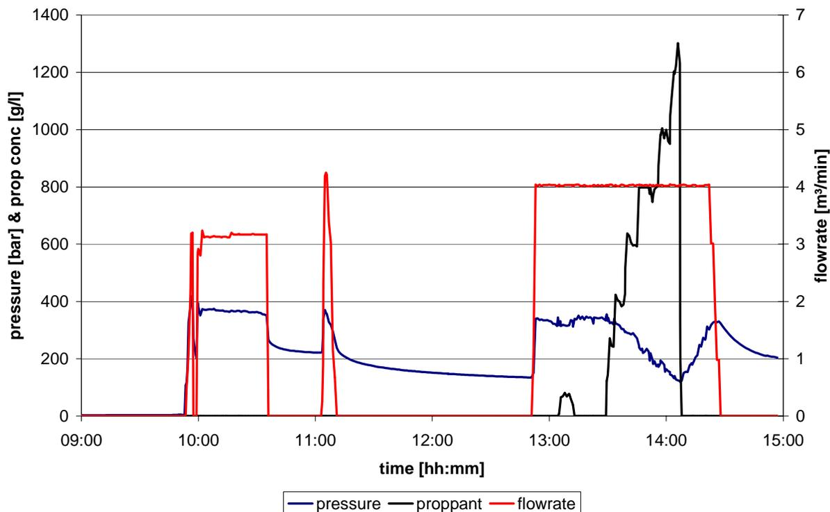
Figure 4 Schedule of the gel-proppant treatment in the Lower Dethlingen sandstones starting with a leakoff test and a step-rate test.
