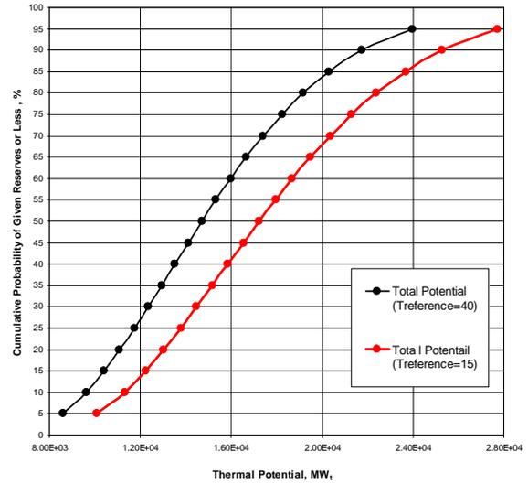
Figure 4. Cumulative frequency graph of total thermal energy power potential of major geothermal fields in Turkey with different reference temperatures.
