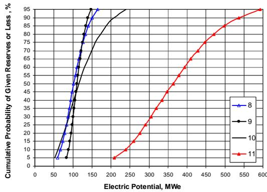
Figure 2. Cumulative frequency graph of power generation potential of four major geothermal fields in Turkey.
