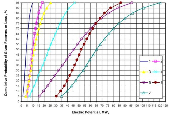
Figure 1. Cumulative frequency graph of individual power generation potentials of seven geothermal fields in Turkey.
