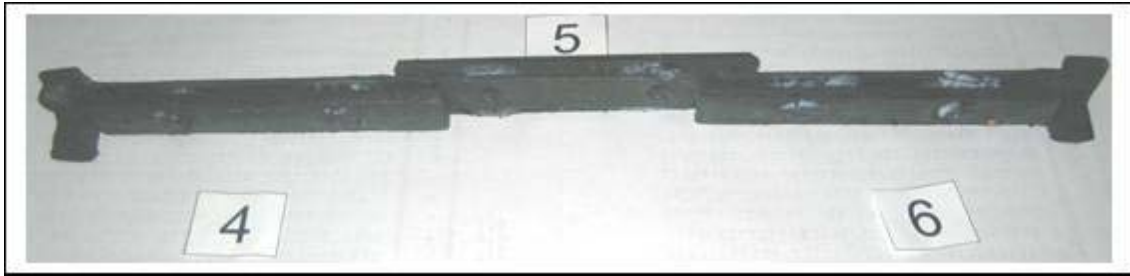
Figure 4. Metal coupons 4 – 6, ~150°C, acidified pH ~4.5
