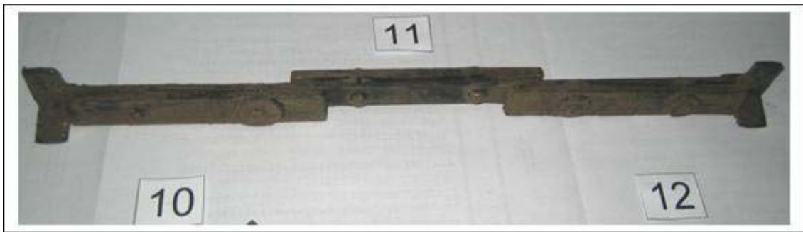
Figure 6. Metal coupons 10 – 12, ~120°C, acidified pH~4.5 and with corrosion inhibitor
