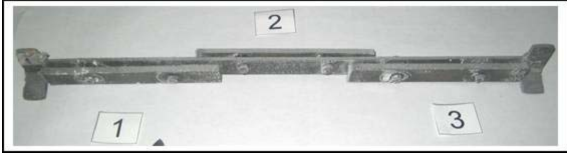
Figure 3. Metal coupons 1 – 3, blank/reference line condition, ~160°C, un-acidified
