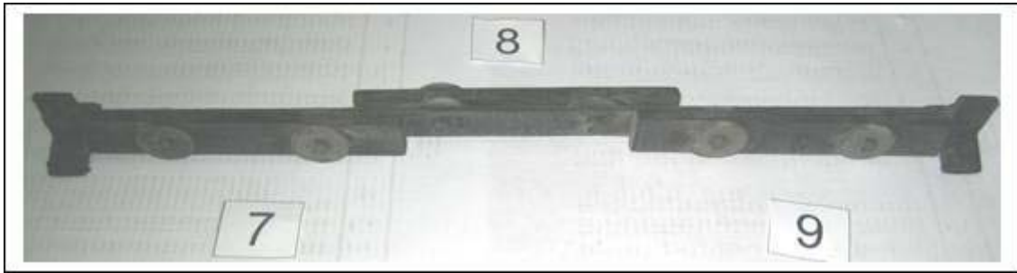
Figure 5. Metal coupons 7 – 9, ~120°C, acidified pH ~ 4.5
