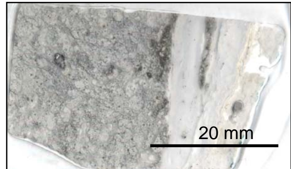
Figure 1. Example of thick section of vein and hostrock: sampled from 226' in Steamboat 87-29 exhibiting grey quartz and milky white quartz in vein fracture, propylitic alteration, and strong siliceous alteration of matrix.
