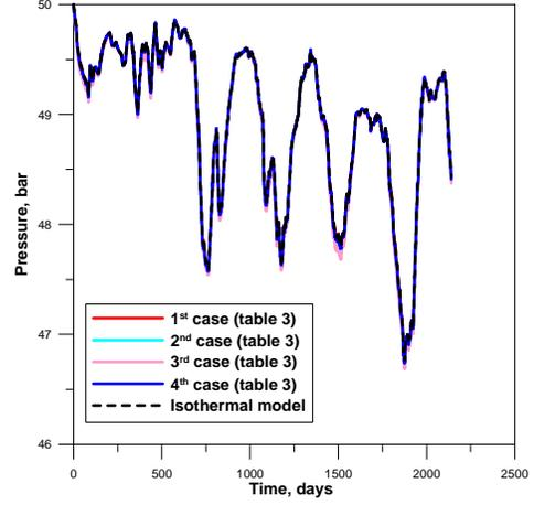
Figure 13: Effects of  $V_r$ ,  $\phi_i$  and  $c_r$  on pressure.
