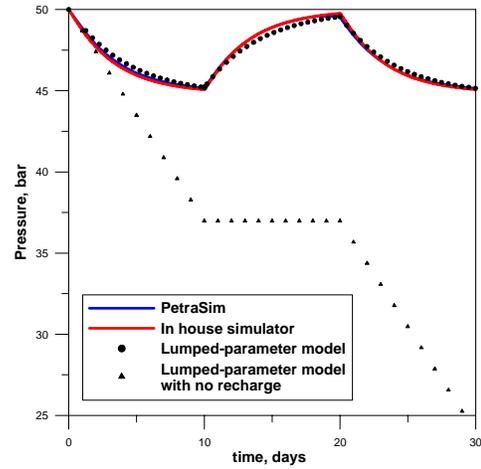
Figure 6: Comparison of PetraSim, our in house simulator, lumped parameter model and the lumped parameter model without recharge for pressure.
