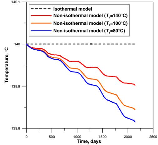
Figure 10: The effect of the recharge temperature on reservoir temperature for  $T_s=80, 100$  and  $140^\circ\text{C}$ .
