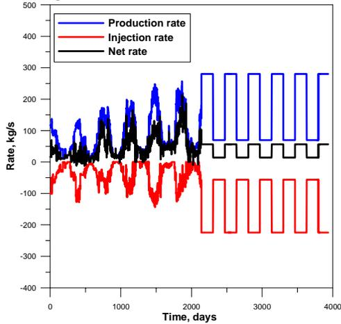
Figure 16: Rate scenario 1 – The reinjection to production ratio is %80.
