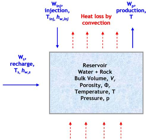
Figure 1. Idealized one tank non-isothermal lumped parameter model.
