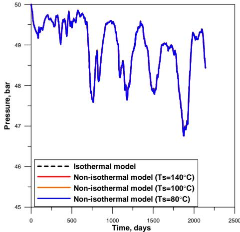
Figure 9: The effect of the recharge temperature on pressure for  $T_s=80, 100$  and  $140^\circ\text{C}$ .
