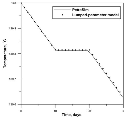
Figure 4: Comparison of PetraSim and the lumped-parameter model for temperature.
