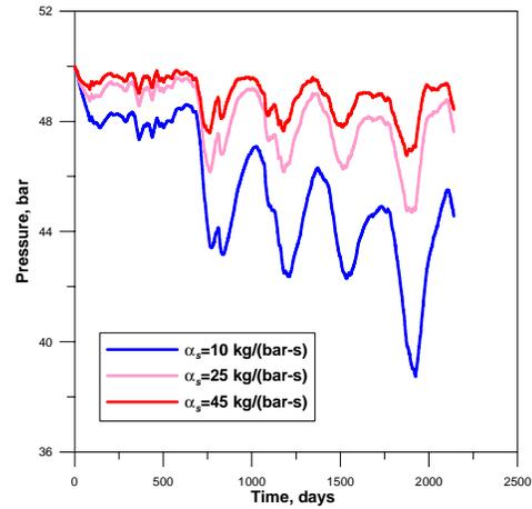
Figure 11: The effect of the recharge index  $\alpha_s$  on the pressure.
