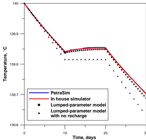
Figure 7: Comparison of PetraSim, our in house simulator, lumped parameter model and the lumped parameter model without recharge for temperature.
