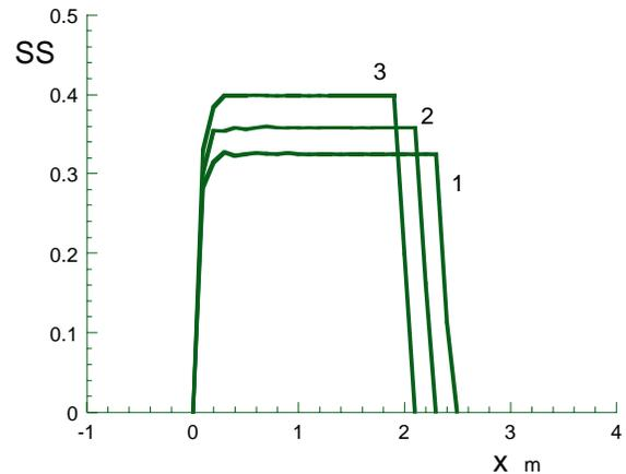
Figure 2. Solid salt distribution after 10 years of production for different initial reservoir pressure. 1 –  $P_0 = 1.4 \cdot 10^7 \text{ Pa}$ . 2 –  $P_0 = 1.5 \cdot 10^7 \text{ Pa}$ . 3 –  $P_0 = 1.6 \cdot 10^7 \text{ Pa}$ .
