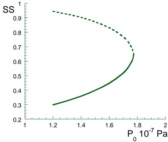
Figure 1. Bifurcation diagram of the similarity solution: solid saturation versus reservoir pressure. Dashed line corresponds to the unstable branch of the solution.  $\phi = 0.1$ ,  $k=0.5 \cdot 10^{-17} \text{ m}^2$ ,  $T_0=513.15 \text{ K}$ ,  $P_w = 2 \cdot 10^6 \text{ Pa}$ .
