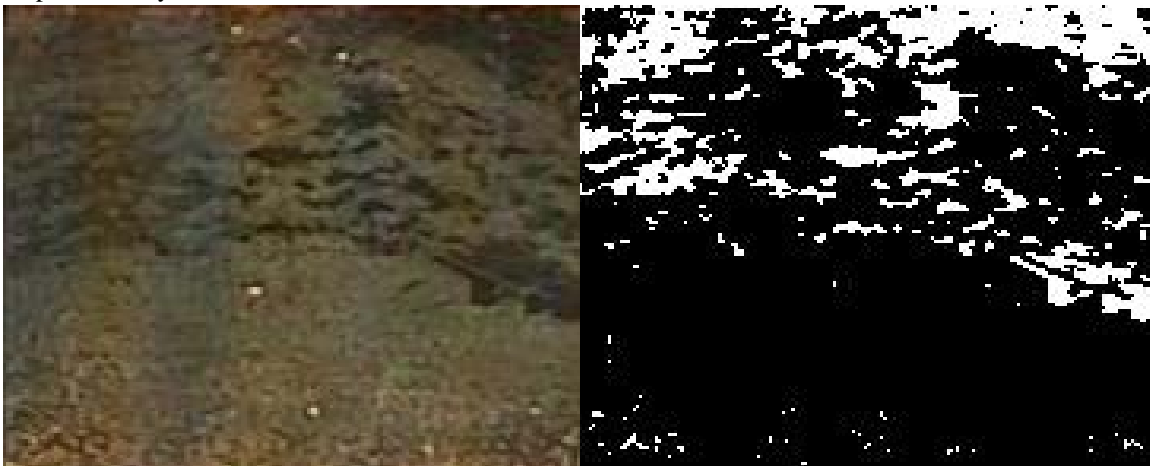
Figure 3. Sample images showing corresponding color and binary images. The light phase is water and the dark phase is gas in the color image. In the binary image, the black is water and the white is gas.
