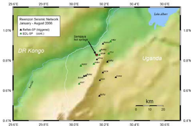
Figure 2. Map showing the distribution of stations. Note, when project started in April 2005 only 3 sites had been occupied. By and by the number was increased to 15 stations.
