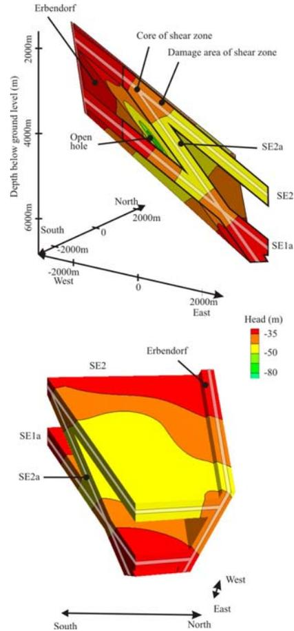
Figure 4 Three dimensional combination of the geomechanical facies at the KTB site, [McDermott, et al., 2006a].
