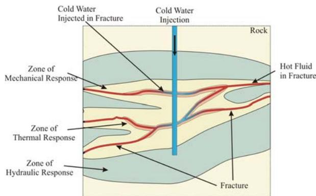
Figure 1 Different processes operate at different scales, example for hydraulic, mechanical and thermal processes.
