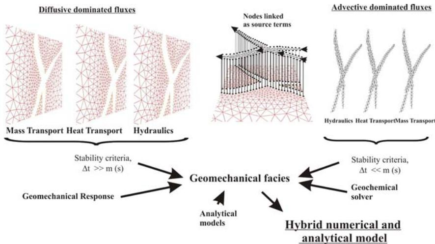
Figure 8 Conceptual illustration of a multiple mesh hybrid numerical analytical model for HTMC coupling based on the geomechanical facies approach
