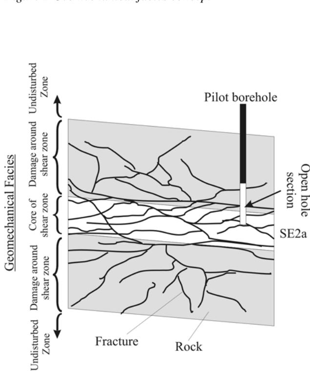
Figure 3 Example of the application of geomechanical facies, after [McDermott, et al., 2006a].
