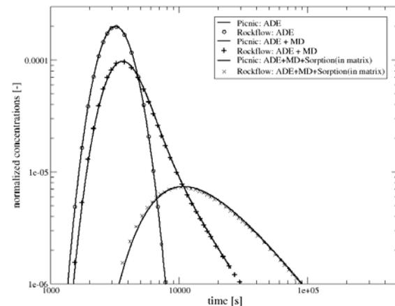
Figure 6 Validation of advection, advection and matrix diffusion, advection matrix diffusion and linear sorption.
