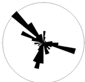
Figure 7. Rose diagram showing joint orientations near CHS resort (Thorum, 2005). n=124 .
