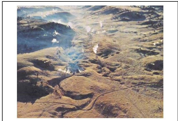
Figure 1. Surface effects (steam and smoke) of an underground coal mine fire near Sheridan, Wyoming (Dunrud and Osterwald, 1980). Note tire tracks for scale.
