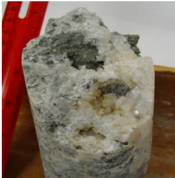
Figure 4. An example of calcite crystals containing much abundant space in the core.
