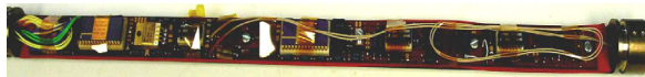
Figure 7 is a photograph of the HT SOI electronics used in the downhole tool.
