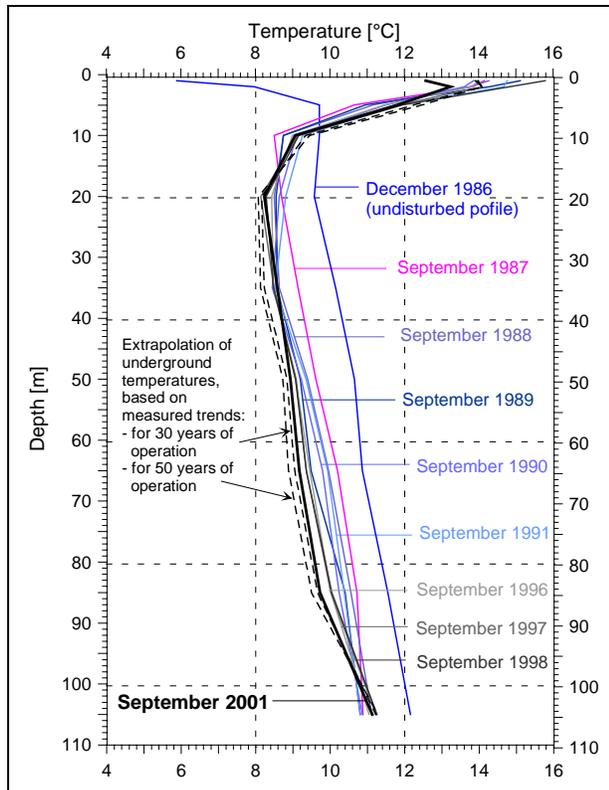
Figure 1. Measured ground temperature profiles at a distance of 1m from the BHE in Elgg. Curve "December 1986" marks the undisturbed profile at the start of the first heating season. The subsequent curves show the conditions after winter heat extraction and summer recovery, just before the start of the next heating season. For extrapolations into the future see text.
