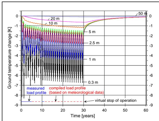
Figure 5. Simulated ground temperature changes of the BHE at Elgg relative to the undisturbed situation in December 1986 over 30 years of operation and 30 years of recovery.
