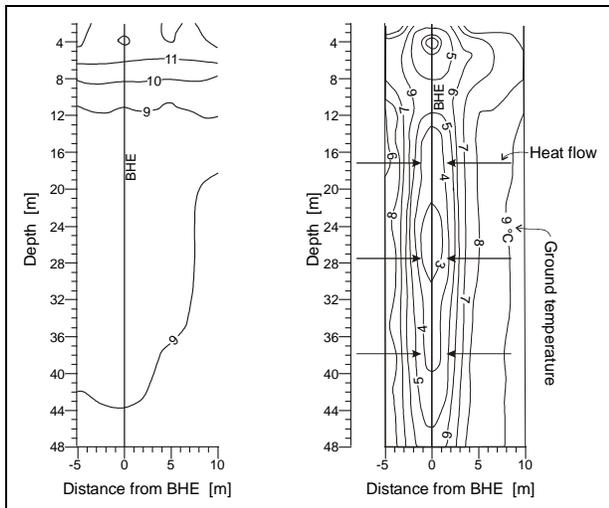
Figure 3. Measured temperature distribution in the ground at the beginning of the monitoring period (left, on 1.10.1986, after a total of ca. 2 hours of test operation) and at the end of the first heating season (right, on 1.5.1987), Schwalbach GSHP test plant, Germany (after RYBACH and SANNER, 1999).
