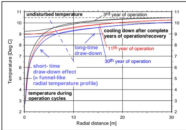
Figure 2. Funnel-like temperature distribution and long term cooling-down around a BHE. The short term and the long term influences are well documented.
