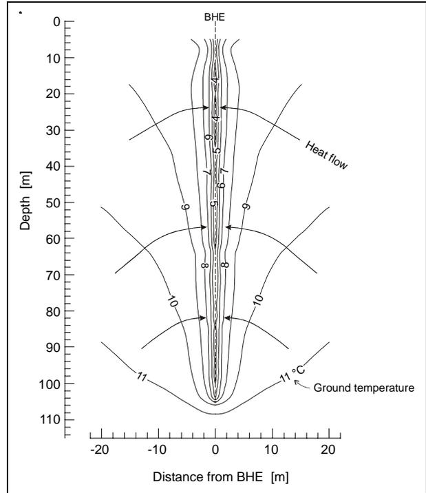
Figure 4: Calculated temperature isolines around a 105 m deep BHE, during the coldest period of the heating season 1997 in Elgg/ZH, Switzerland. The radial heat flow in the BHE vicinity is around 3 W/m<sup>2</sup>.
