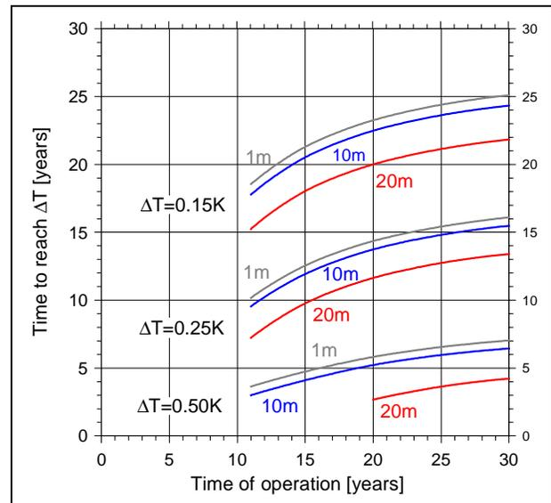
Figure 6. Duration of recovery period to reach a minimal final temperature deficit ( $\Delta T$ ) of 0.5, 0.25 and 0.15K for different distances from the BHE as a function of the time of operation.
