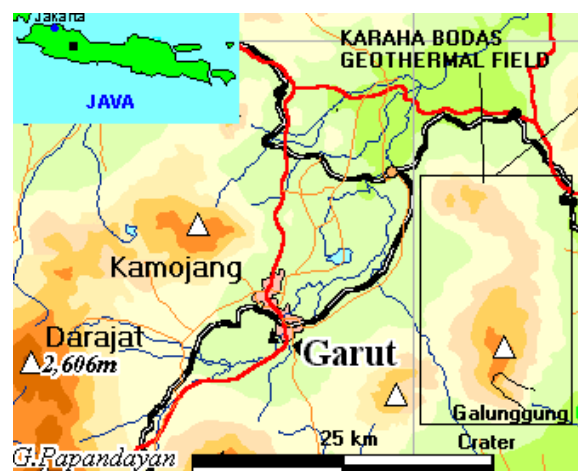
Figure 1. Location Map of the Karaha Bodas Geothermal Field. Darajat (55 MW) and Kamojang (140 MW) are vapor-dominated reservoirs.
