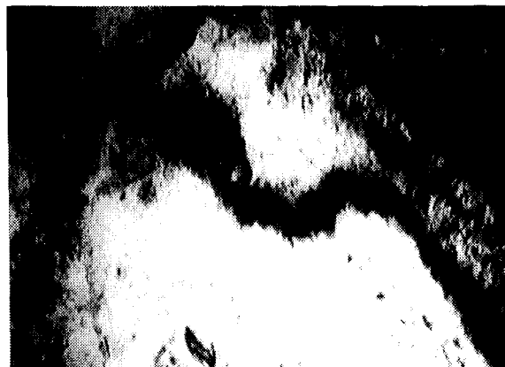
Fig. 3. Corroded growth zone, outlined by fluid inclusions, within the interior of quartz from SB-15-D-430 m. Field of view is 2.2 mm.
