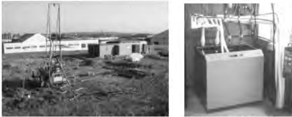
Fig. 2: left: Schwalbach GSHP research station, with light drilling rig, borehole field and buildings for HP and monitoring; photo from January 1988 right: Direct Expansion experiments in Schwalbach GSHP research station in 1989; note ice development on evaporator pipes leading to special BHE
