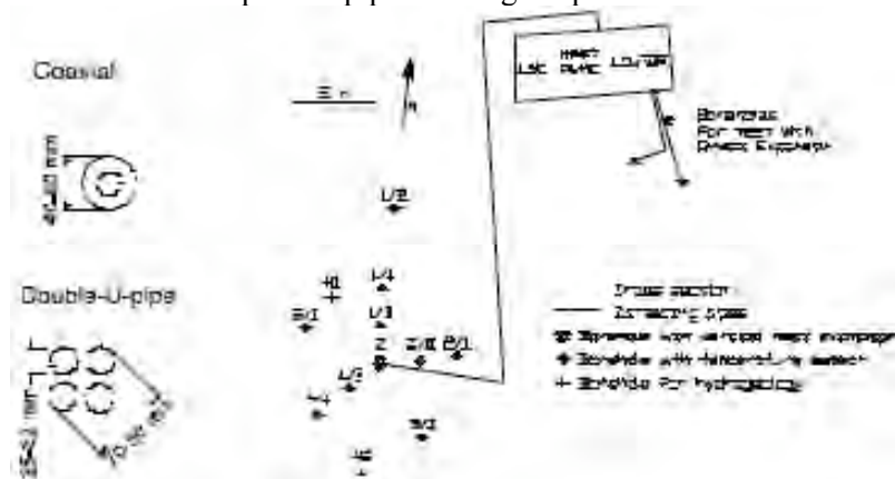
Fig. 3: left: Cross-section of typical BHE, as used in Schwalbach right: Schematic plan of the test plant in Schwalbach
