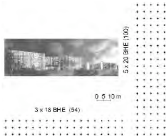
Fig. 13: Layout of the two BHE fields for the office building in Langen, with the architect's impression of the building to show its location in regard to the BHEs
