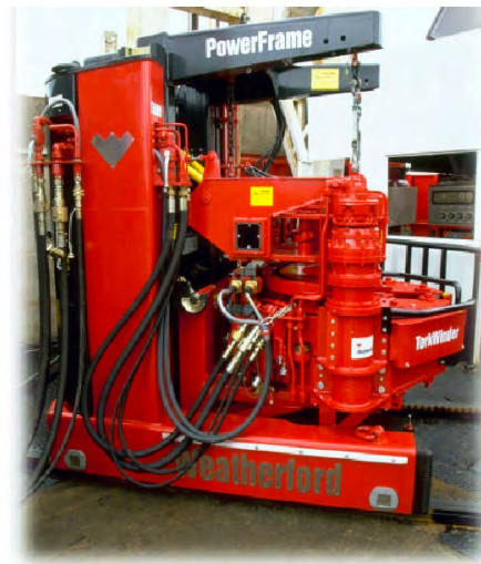
Figure 5: Iron roughneck offshore
