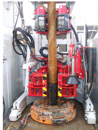
Figure 6: Iron roughneck onshore
