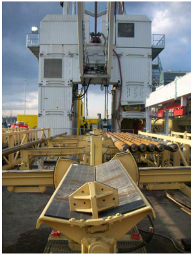
Figure 3: Horizontal pipe rack
