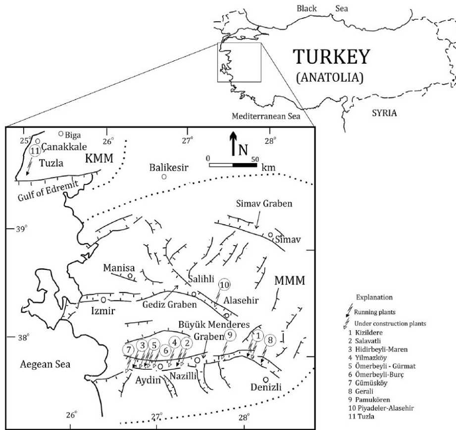
Figure 1: Distribution of locations with geothermal resources suitable for electricity generation and power plants in Turkey.
