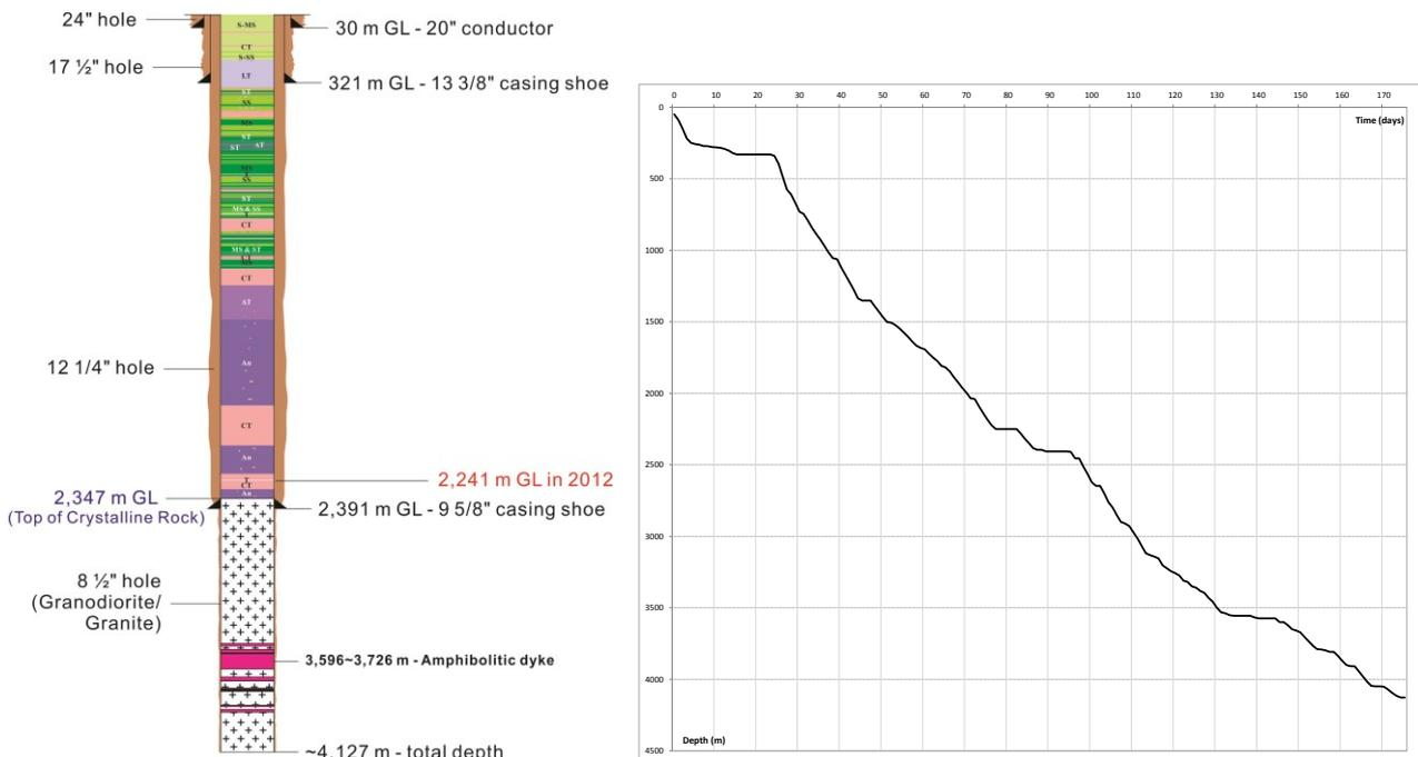
Figure 3. Geologic sequence as a result from mud logging superimposed with well specification (left) and merged drilling depth versus time plot (right).
