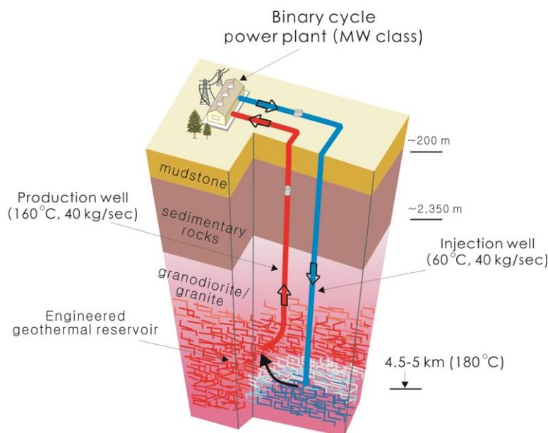
**Figure 1. Conceptual model of the Korean EGS pilot plant project.**
