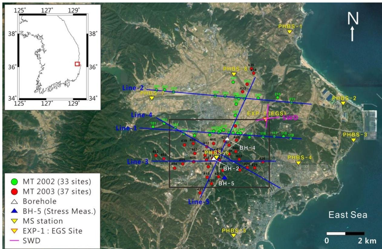
**Figure 2.** Location map of the Pohang site showing MT measurements, major wells, geophone lines for seismic-while-drilling (SWD), and nine MS monitoring stations (PHBS-1~8 and EXP-1). Boreholes BH-1 and BH-3 are in close vicinity of BH-2 and BH-4, respectively, so are omitted for the sake of simplicity. Note that EXP-1 is located at EGS drilling site.
