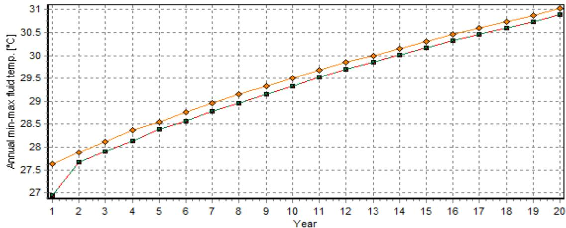
**Figure 7: Fluid temperature in BHEs system during 20 year of operation**
