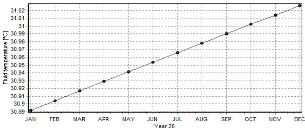
**Figure 6: Fluid temperature in BHEs system in 20<sup>th</sup> year of operation**
