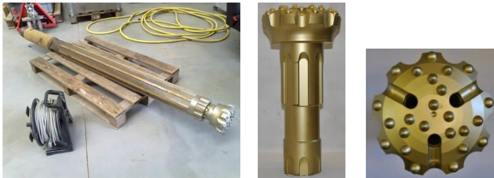
Figure 4: configuration of the DTH water hammer BHA including the 6 inch Wassara W-150 hammer and the 7 ¼ inch drill bit designed by GZB, clearly visible are the guiding ribs on the hammer housing (left) for high accuracy.
