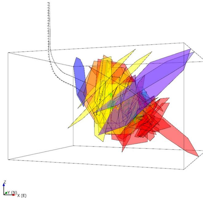
**Figure 1: The 131 discrete fractures included in the Utah FORGE 2025 v1 DFN. Colors of fractures indicate identification order with respect to well 16A(78)-32 stimulation stage (Finnila, 2025).**
