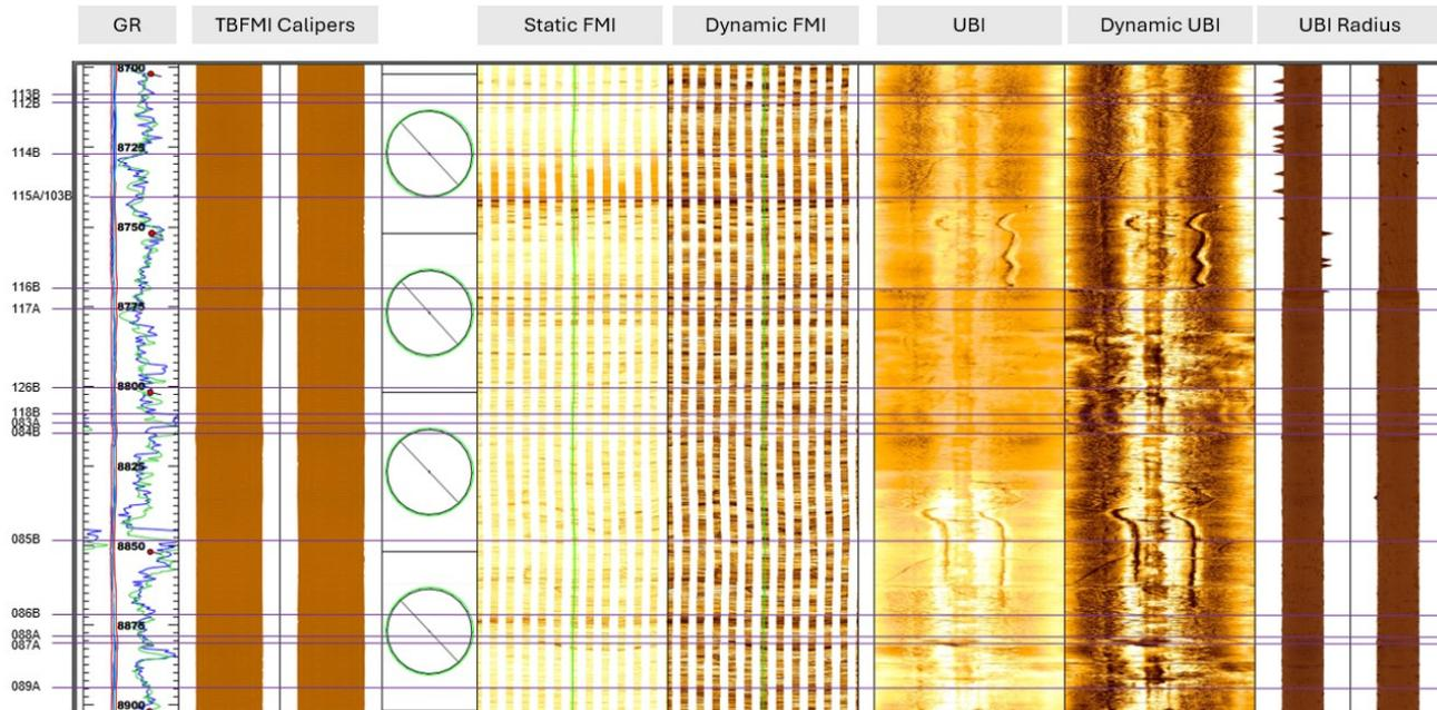
Figure 15: Section of FMI and UBI logs for well 16B(78)-32 showing locations of intersections with DFN fractures (purple lines). Short fracture names included as labels on the left side of figure. Log image from file “Univ of Utah Forge 16B-78-32 TBFMI-UBI Trip3 TOH 6252-10914 5in.pdf” included in GDR release May and Jones (2023).
