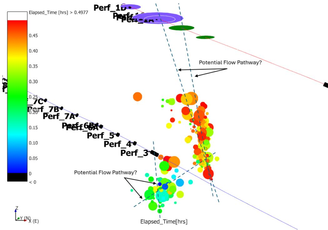
Figure 7: Microseismic points recorded during the first 30 minutes of the stimulation of Stage 3 in well 16A(78)-32 suggest two or more fractures may be creating flow pathways between the wells (MEQ data from Dyer et al, 2023).
