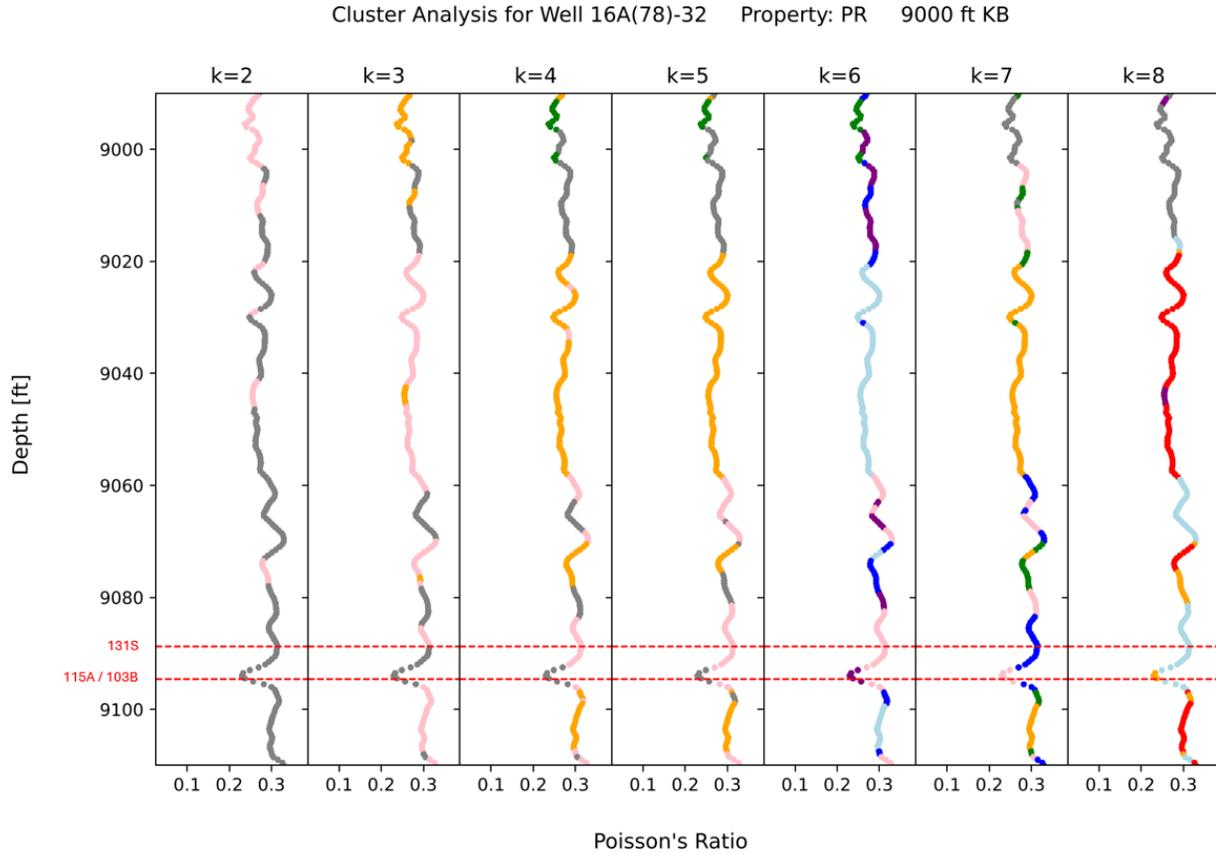
**Figure 17: Cluster analysis results for well 16A(78)-32 at k values between 2 and 8 showing Poisson’s ratio acoustic log values at depths between 9000 ft and 9100 ft along with the intersection points of DFN fractures (dotted red lines). Poisson’s ratio log data from Gilmour et al., 2021.**
