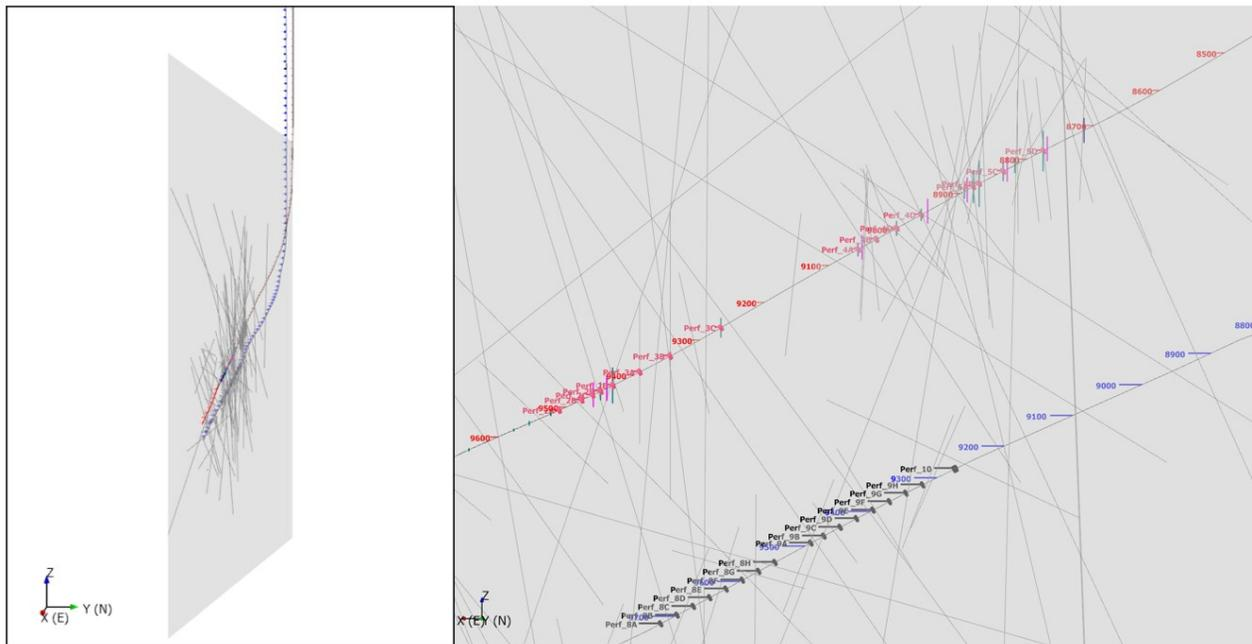
**Figure 18: DFN fracture traces (grey lines) on a vertical plane aligned with wells 16A(78)-32 and 16B(78)-32. Pink and green vertical bars on 16B(78)-32 show locations of interpreted frac hits. Note that fracture locations are somewhat approximate as the vertical trace plane cannot align exactly with the entire length of the well trajectories.**
