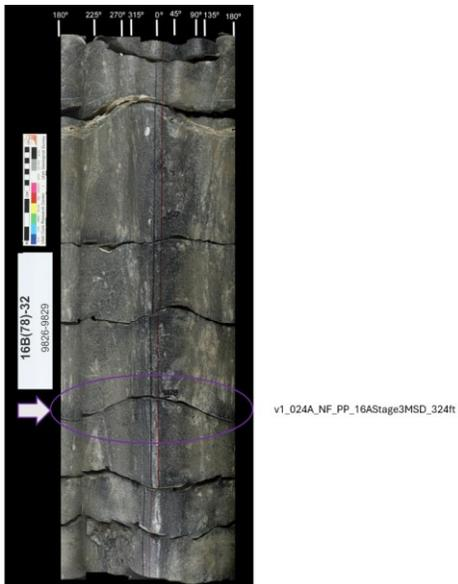
**Figure 12: Core sample from well 16B(78)-32 showing fracture matching DFN fracture v1\_024A\_NF\_PP\_16AStage3MSD\_324ft. Core photo from Jones (2025). Note that location of core fracture has been shifted 13.1 ft from this photo label based on analysis by Jones et al. (2025) so the fracture intersection depth on 16B(78)-32 is assumed to be 9841.15 ft MD KB.**
