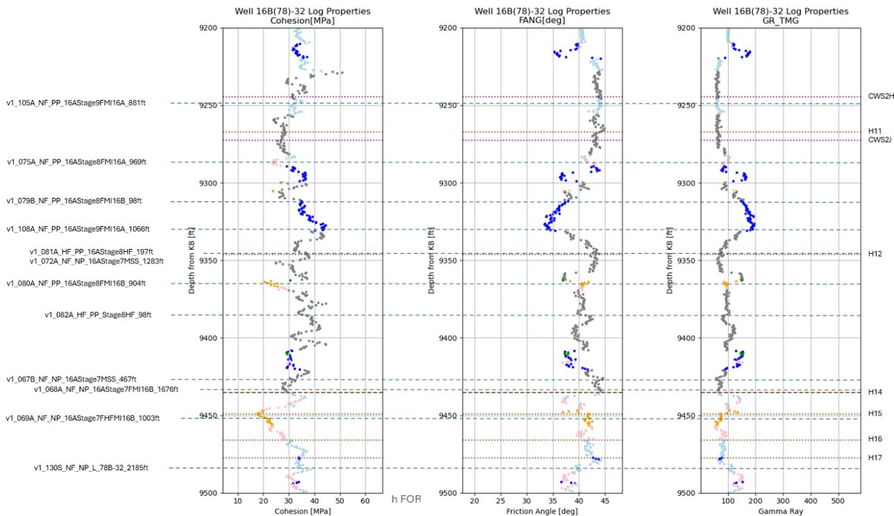
**Figure 19: Correlation of the DFN with frac hit locations and sonic log data on well 16B(78)-32. Colors show the k-means clustering results (k=6) of the analysis performed on the sonic log data to highlight differing rock types. Fracture ids are shown on the left side of the figure (blue dotted lines) while frac hit identifiers are shown on the right side (brown and purple dotted lines). Log data is from May and Jones, 2023.**
