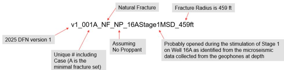
**Figure 2: Example showing parts of the DFN discrete fracture naming convention.**
