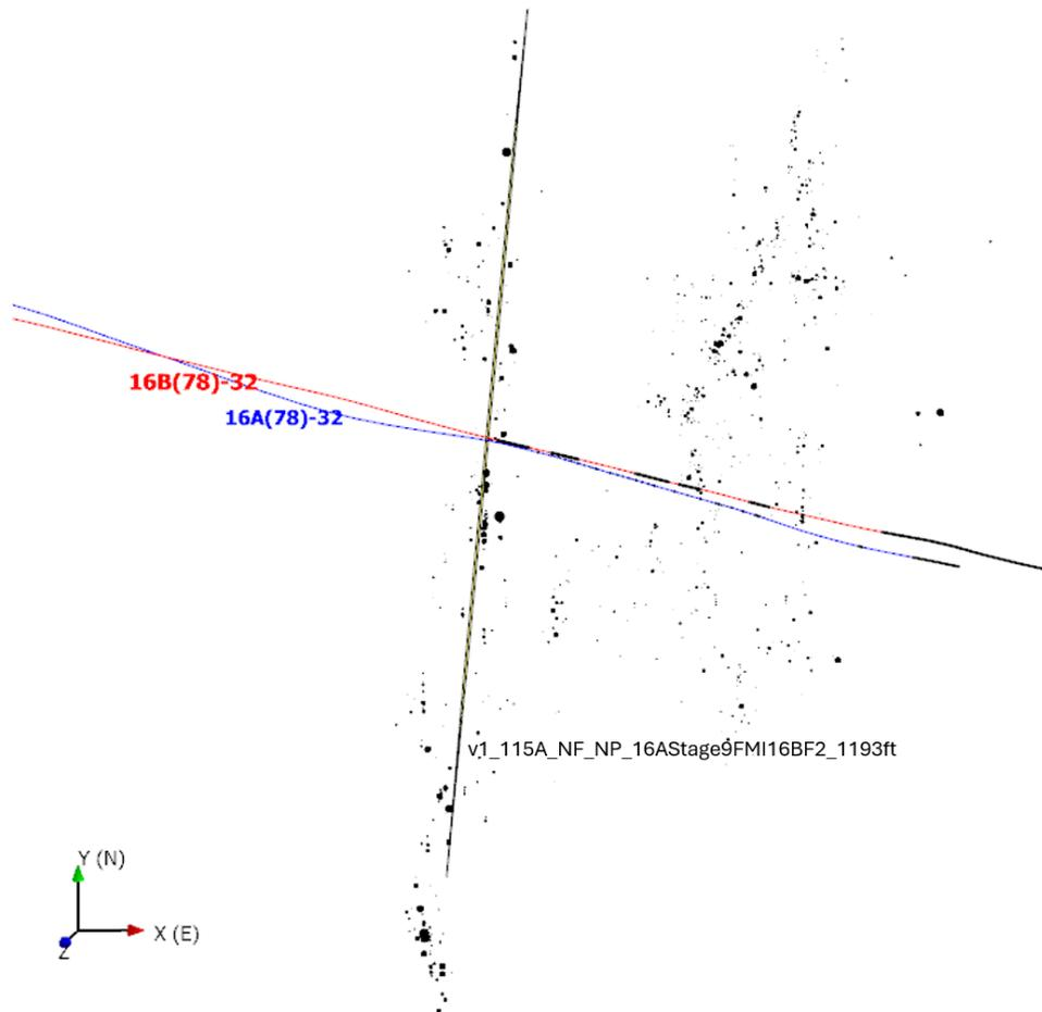
**Figure 14: Top-down view of Niemz et al. (2024) microseismic data with one of the DFN fractures** Microseismic points sizes are scaled by magnitude. Open hole and stimulation stages are shown in black on well 16A(78)-32 and 16B(78)-32 boreholes.
