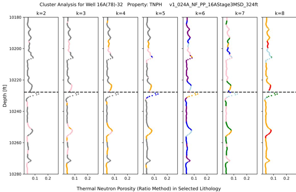
**Figure 10: Cluster analysis results for well 16A(78)-32 at k values between 2 and 8 showing the thermal neutron porosity measurements surrounding the intersection point of fracture v1\_024A\_NF\_PP\_16AStage3MSD\_324ft (dotted line).**
