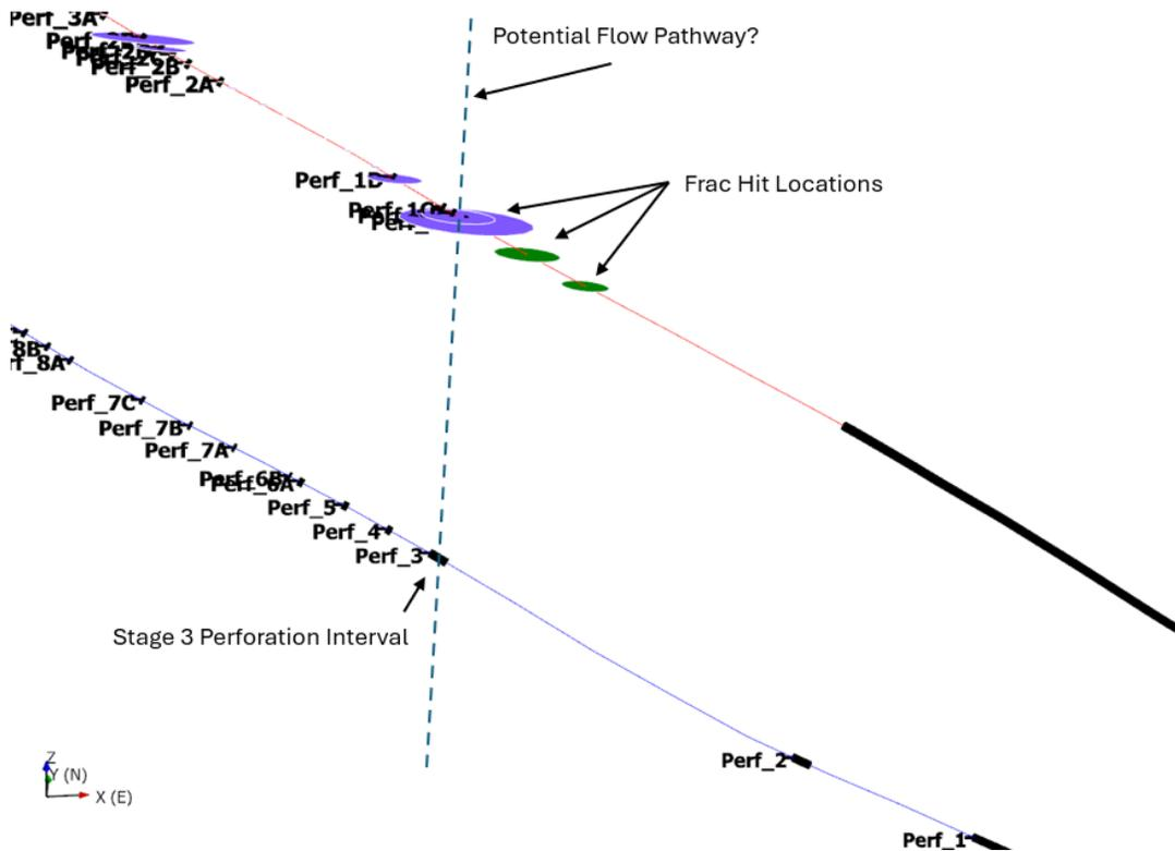
**Figure 5: Starting workflow to find fractures for flow pathway created during stimulation of Stage 3 in well 16A(78)-32.**
