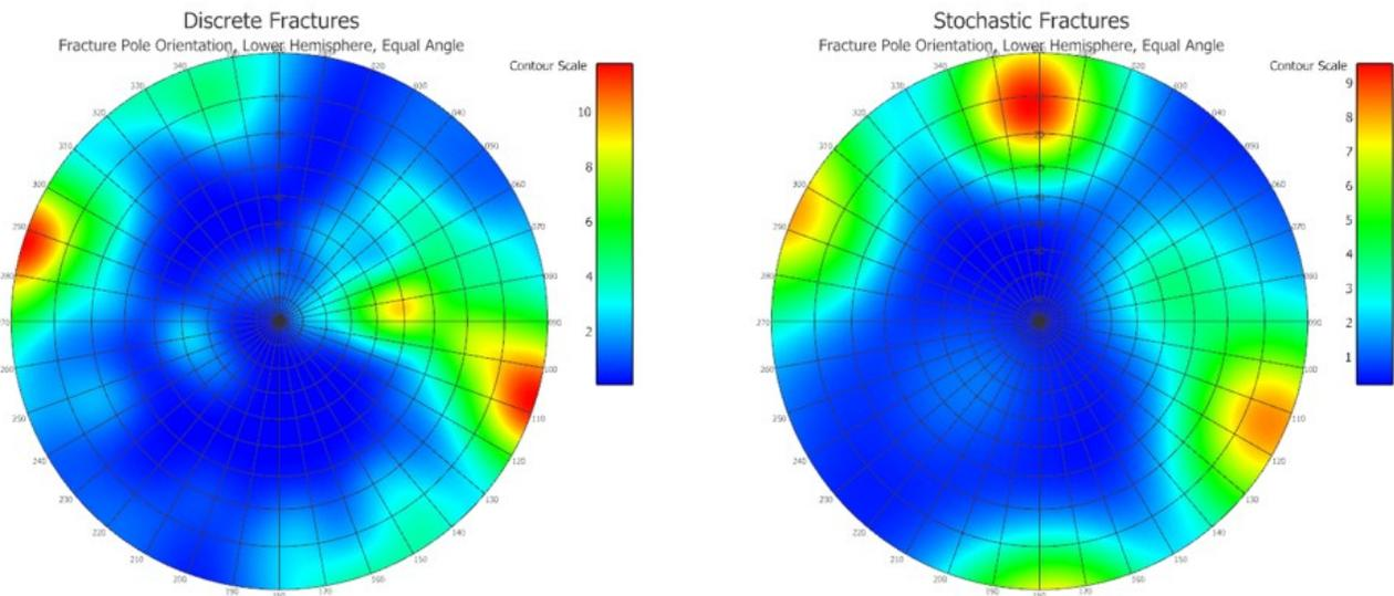
**Figure 4: Contour stereonet plots showing orientations of the discrete and stochastic fractures included in the DFN.**
