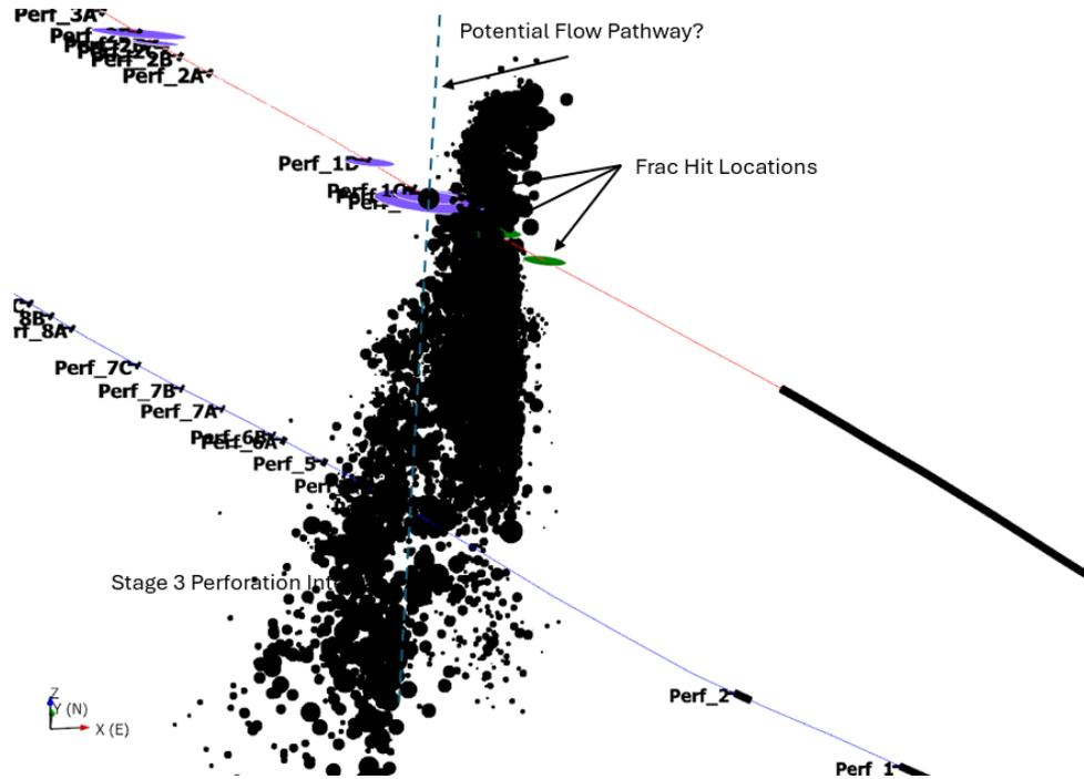
Figure 6: Microseismic point cloud recorded during the 2022 stimulation of Stage 3 in well 16A(78)-32 (MEQ data from Dyer et al, 2023).
