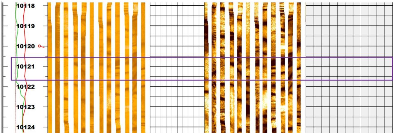
Figure 8: FMI log image showing the location of a Handwerger interpreted fracture in the Stage 3 perforation interval for well 16A(78)-32 (image from Gilmour et al., 2021).
