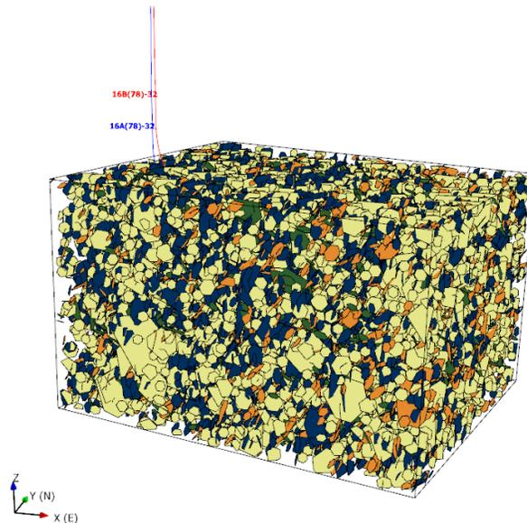
Figure 3: Stochastic fractures included in the Utah FORGE 2025 v1 DFN (Finnila, 2025).
