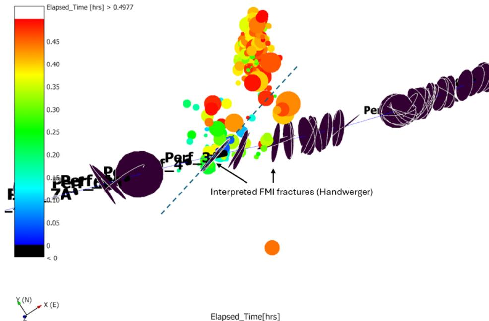
Figure 9: Handwerger interpreted FMI fractures along the borehole of well 16A(78)-32 (black discs show orientations). Microseismic point locations recorded during the first 30 minutes of stimulation of Stage 3 shown in color.
