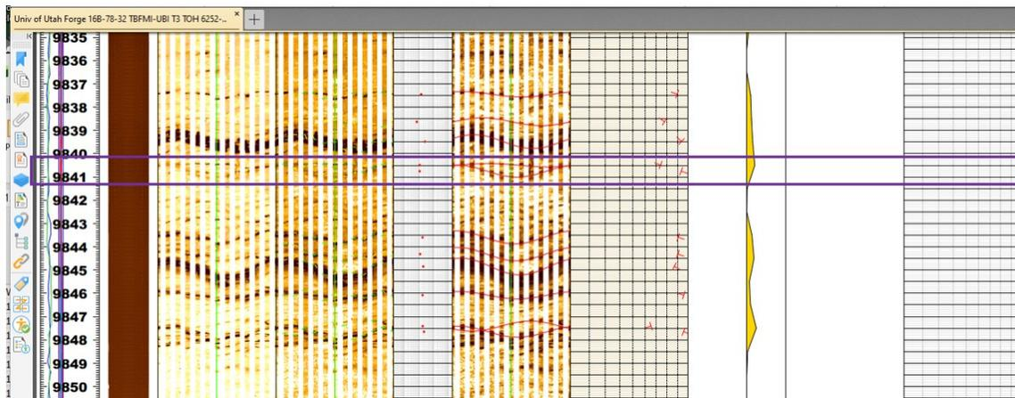
**Figure 11: Interpreted FMI log for 16B(78)-32 at the intersection depth with fracture v1\_024A\_NF\_PP\_16AStage3MSD\_324ft outlined in purple (image from May and Jones, 2023).**
