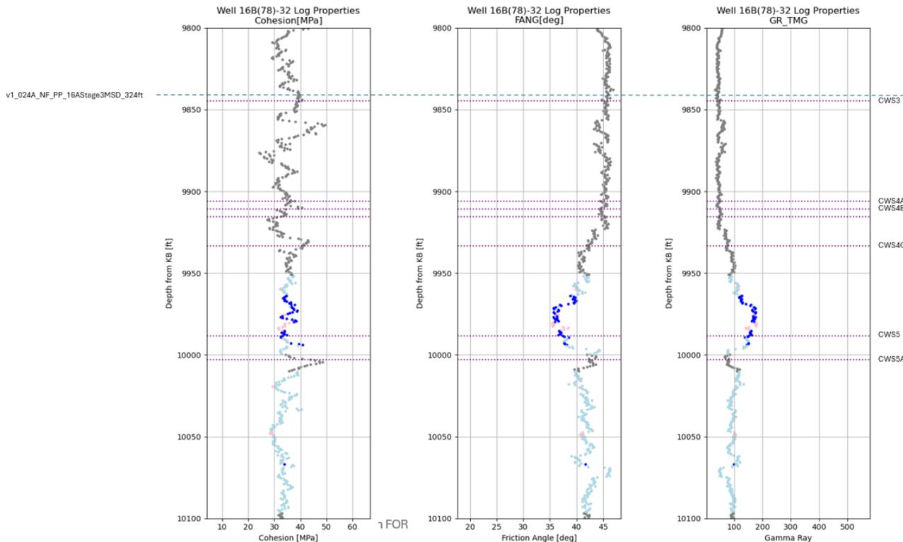
**Figure 13: Correlation of the DFN fracture, v1\_024A\_NF\_PP\_16AStage3MSD\_324ft (blue dotted lines), with frac hit locations and sonic log data on well 16B(78)-32. Colors show the k-means clustering results (k=6) of the analysis performed on the sonic log data to highlight differing rock types. Frac hit identifiers are shown on the right side of the figure with brown and purple dotted lines indicating depths.**
