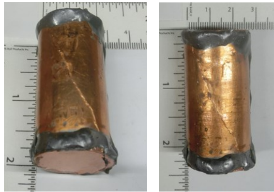
Figure 8: Distinct trace of a well-developed shear fracture marked on the copper jacket after rock failure.
